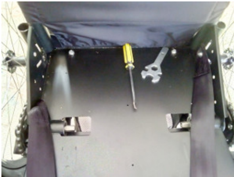
Figure 15: Moving the provided seatbelt to the furthest forward of GRIT's various predrilled anchor points. Boonwurrung Country, April 2022.
